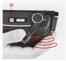
By winding the film advance lever until it stops, the figure "1" will appear in the exposure counter (39), the red mark indicating incomplete film winding will disappear, and the film will be positioned for the first exposure
