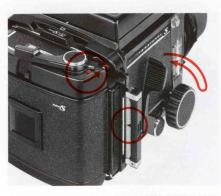
When the shutter is cocked, the dark slide is slightly pulled out (approx. 1/4 in.) and the shutter release button is pressed, the shutter can be released without exposing the film in the roll film holder to light. This operation can be utilized for shutter testing prior to photographing.
