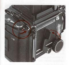
When the multiexposure lever of the roll film holder is moved forward, the coupling pin for double-exposure prevention is disengaged, and whenever the shutter cocking lever is set, shutter releasing can be repeated without limit.
