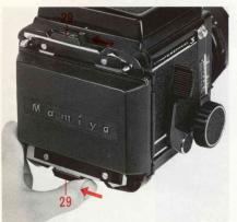
By moving the slide locks (29) on both sides fully to the left, the cap can be removed.
