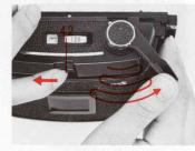
When the film advance lever is continuously wound, with the film wind-stop release lever (42) pushed to the left, the film can be reeled up completely to its end, even though picture taking is still in progress and a film remains unexposed.
