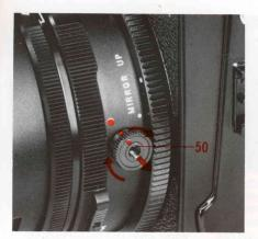
In mirror-up photography, previously release the mirror and operate only the lens shutter at the moment of taking the photograph.
