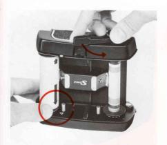
Move the film advance lever gently, until the starting mark (arrow) of the leader paper aligns with the starting mark of the holder. The film advance lever can be moved in several short, definite strokes.
