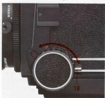
After adjusting the focus, turn the focusing knob fixing lever (18) forward and appropriately clamp it, whereby the focusing mechanism is secured.
