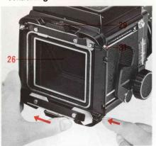
Before attaching the holder, confirm that the upper and lower side slide locks (29) are on the left end of the indented portion when viewed from behind the camera body.
