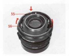
It is advisable to release the shutter when the lens is not to be used for a long period. To release a lens shutter which is removed from the camera body, turn the cocking pins (56) clockwise, while pressing the shutter lock pin (55) with a finger. The cocking pins should be turned all the way; do NOT leave the pins turned only halfway.
